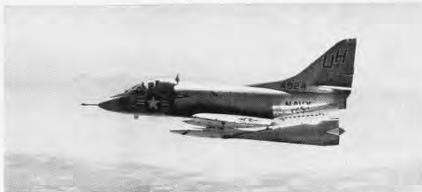
AT NAS Miramar recently, Commander Bernard Tesch, Jr., VC-7, made the first flight of an A-4 carrying a center-of-gravity-towed Dart target. Improved tow and suspension equipment allows the target to remain completely clear of the runway during takeoff. Once airborne, a one-way tow reel streams the target approximately 2,000 feet behind the Skyhawk. Previously the maneuverable target was snatched off the ground or dragged on the runway during takeoff.
